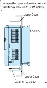
Mounting the External Heatsink Ventilation Space
