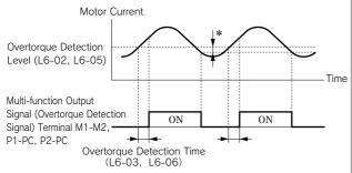
\* The releasing width of overtorque detection is approx. 10 % of the inverter rated current (or motor rated torque).
