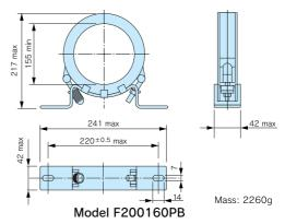
Can be used both for input and output sides of the inverter and effective on noise reduction.
