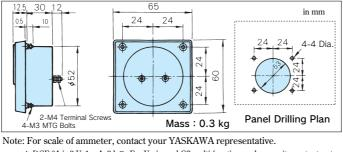
\* DCF-6A is 3 V, 1 mA, 3 k  $\Omega.$  For Varispeed G7 multi-function analog monitor output, set frequency meter adjusting potentiometer or constant H4-02, -05 (analog monitor output gain) within the range of 0 to 3 V (initial setting is 0 to 10 V).
