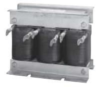
When power capacity is significantly greater when compared to inverter capacity, or when the power-factor needs to be improved, connect the AC or DC reactor.
