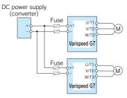
Note: When connecting multiple drives together, make sure that each drive has its own fuse. If any one fuse blows, all fuses should be replaced.
