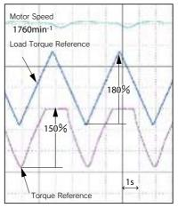
Torque Control (Torque limit set at 150%)
