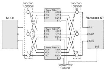
When wiring contactors in parallel, make sure wiring lengths are the same to keep current flow even to the relay terminals. Ground wires for noise filter and inverter should be thick and as short as possible.
