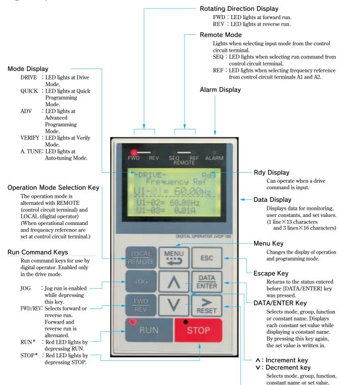
\* RUN or STOP LED turns ON or OFF, or blinks in accordance with each operation.
