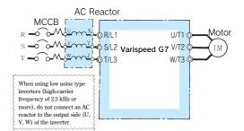
Select an AC reactor according to the motor capacity. Standard Varispeed G7 is a DC reactor.
