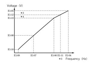
Set E1-04 to 11 so that E1-04 $\geq$ E1-11 $\geq$ E1-06 $\geq$ E1-07 $\geq$ E1-09. To make the line of the V/f characteristics straight, set E1-07 and E1-09 to the same value. At this time, the set value of E1-08 is disregarded.
