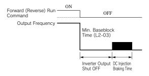
The DC injection braking time is as follows, according to the output frequency when stop command is input.
