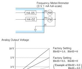
100 % Output Frequency (Inverter Output Current)
